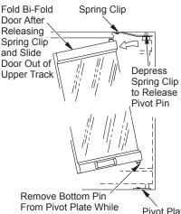
From Pivot Plate While Sliding Door Out of the Upper Track
